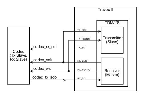
Connections for Codecs with common WS and SCK signals for RX and TX directions
