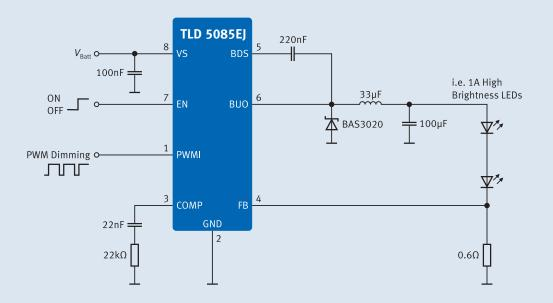
THE TLD 5085EJ IS A SMART LED BUCK driver circuit, that provides all active functions for a constant current switching regulator, capable of delivering up to 1.8A load current with excellent line and load regulation.
