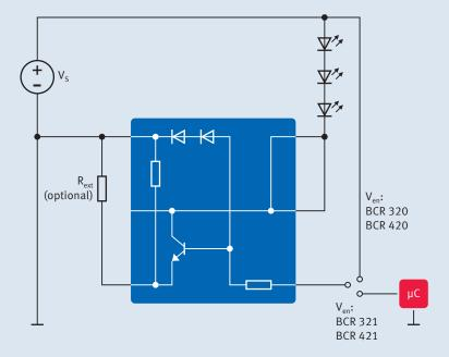
THE BCR 32XU AND BCR 42XU LED DRIVERS are dedicated LED drivers for 0.5W LEDs with a maximum output current of 250mA. They are optimized in terms of cost, size and feature set for medium power LEDs.
