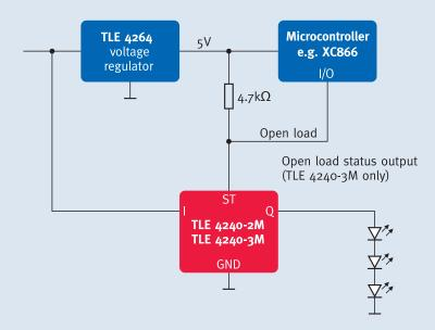
THE TLE 4240-2M/-3M IS A MONOLITHIC integrated, low dropout linear constant current source. It is designed to supply white or color LEDs in order to achieve constant brightness and extended LED lifetime, independent from supply voltage or LED forward voltage class.
