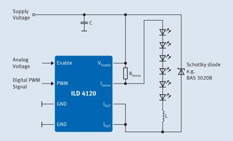
THE ILD 4120 IS A STEP DOWN CONVERTER with integrated power stage in a small thermally enhanced DSO-8 package tailored to drive 3W LEDs.
