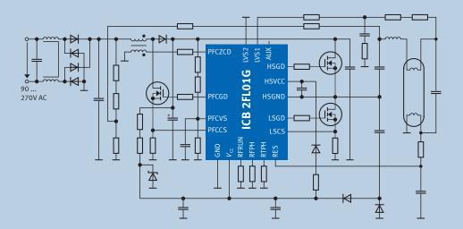
SMART BALLAST CONTROLLER ICB 2FL01G is designed to control a fluorescent lamp ballast including
