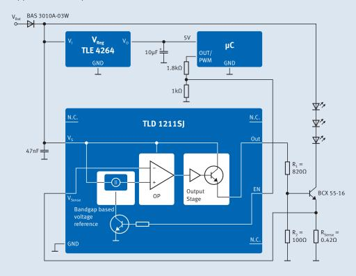
THE TLD 1211SJ IS AN INTEGRATED ADJUSTABLE current source. It is designed to supply LEDs realizing constant brightness and to extended LED lifetime. The TLD 1211SJ is able to drive output current up to 85mA. By using an additional external output stage up to 2.5A for high current LEDs are possible.
