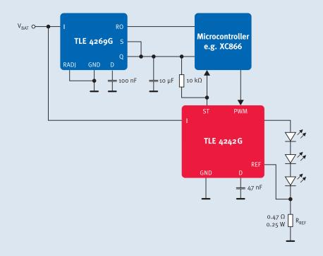
THE TLE 4242G IS AN INTEGRATED ADJUSTABLE constant current source, driving loads up to 500mA. The output current level can be adjusted via an external resistor. The IC is designed to supply high-power LEDs (e.g. Osram Dragon LA W57B) under the severe conditions of automotive applications resulting in constant brightness and extended LED lifetime.
