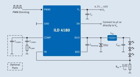
THE ILD 4180 IS A MONOLITHIC INTEGRATED high-brightness LED driver circuit, that provides all active functions for a constant current switching regulator, capable of delivering up to 1.8A load current with excellent line and load regulation.
