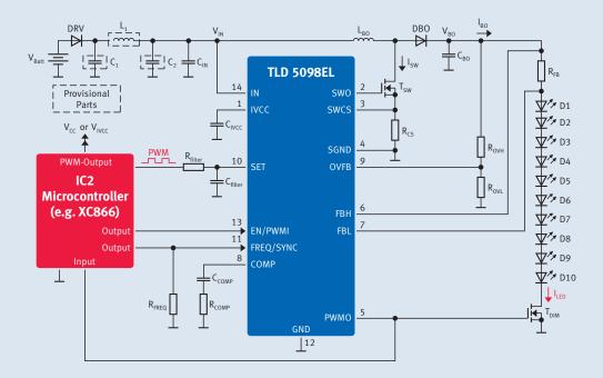
THE TLD 5098EL IS A SMART LED BOOST controller with built-in protection and diagnostic features. The main function of these devices is to step-up (boost) the output voltage and regulate a constant LED current. The device has an implemented analog dimming feature to adjust the average LED current.
