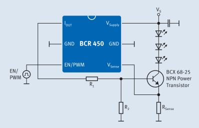
THE BCR 450 IS AN LED CONTROLLER used in combination with a bipolar transistor to drive medium power and high power LEDs.
