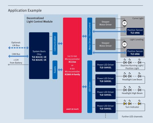
DECENTRALIZED FRONT LIGHT modules are used if the control of light functions is transferred to separate ECUs close to the front light modules. It combines functions to control LEDs and stepper motor control for advanced front light control (AFS). In order to establish AFS functionality, it needs to process information regarding the vehicle speed, steering angle and further vehicle parameters usually distributed via CAN bus.
