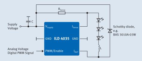
THE ILD 4035 IS A STEP DOWN CONVERTER with integrated power stage in a very small SC-74 package tailored to drive 1W LEDs.
