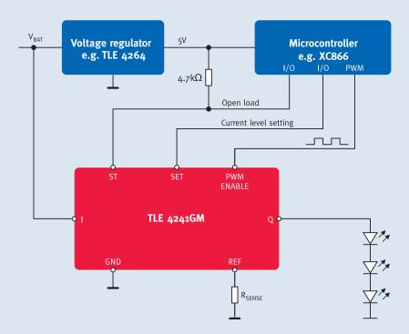
THE TLE 4241GM IS AN INTEGRATED adjustable constant current source, providing an output current adjustable via different means. The IC is designed to supply LEDs under the severe conditions of automotive applications resulting in constant brightness and extended LED lifetime.
