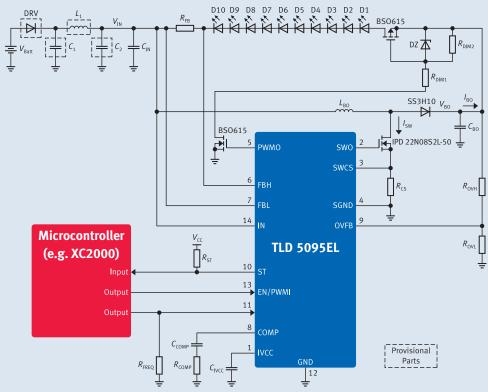
THE TLD 5095EL IS A SMART LED BOOST controller with built in protection and diagnostic features. The main function of these devices is to step-up (boost) the output voltage and regulate a constant LED current. The device has an implemented status pin for diagnostic function.
