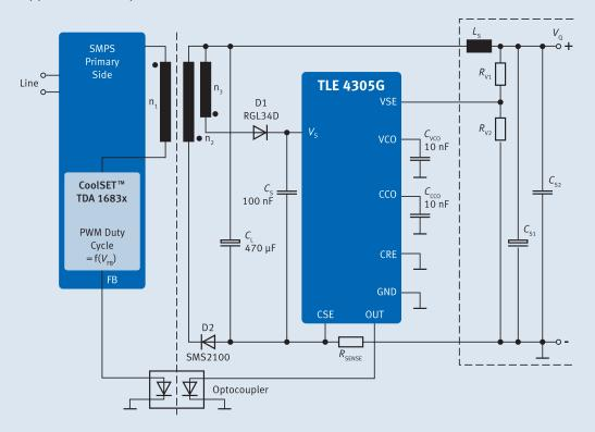
THE TLE 4305G IS SPECIFICALLY DESIGNED to control the output voltage and the output current of a switch mode power supply. Independent compensation networks for the voltage- and for the current-loop can be realized with external circuitry.
