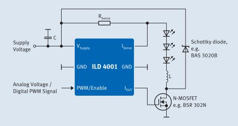
THE ILD 4001 IS A STEP DOWN LED CONTROLLER with external power stage in a very small SC-74 package tailored to drive LEDs with 700mA up to 10A.
