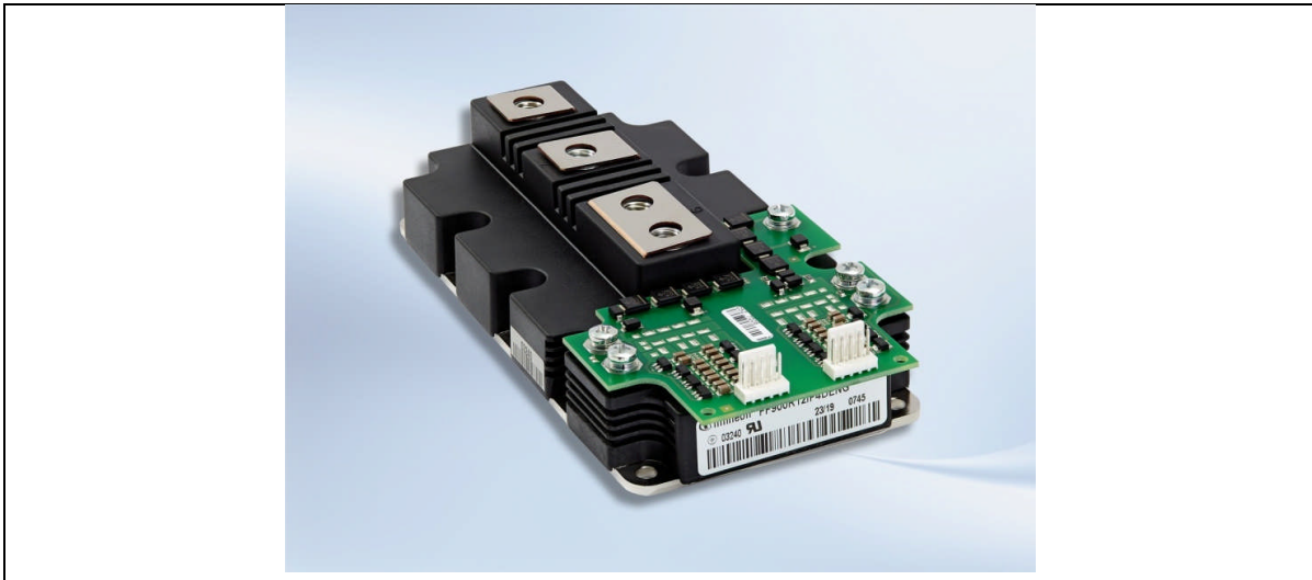
Fig. 21: MA300E12 Adapter Board mounted on a PrimePACK™ 2
