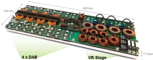
On-board charger: increasing power density from today's 2kW/l to 10kW/l with GaN
