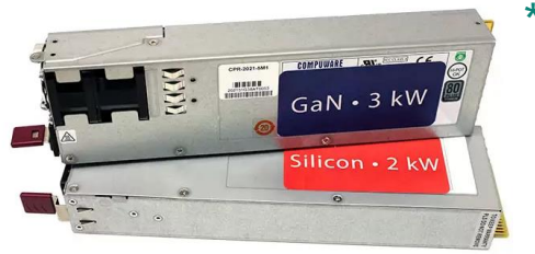
HP-SMPS for server: GaN is enabling highest power density and efficiency, to enable Accelerated- and AI computing at lowest TCO
