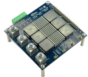
48V to ~7V/1V conversion: with GaN brings smaller form factors to Accelerated- and AI computing as well as Telecom brick converters
