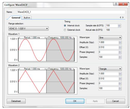
The WaveDAC8 component provides the following parameters.
