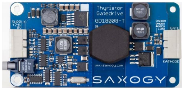
Figure 25. Trigger Circuit GD18008-T for continuous trigger signals
