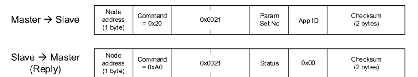
Figure 5 UART Save parameter command = 0x21, Data Word0 = 0x0021
