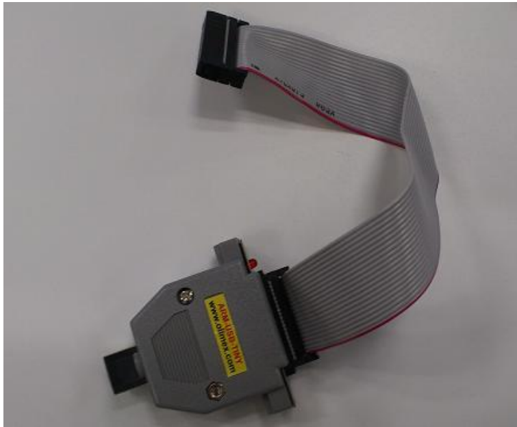
Figure 4. ARM-USB-TINY from olimex
