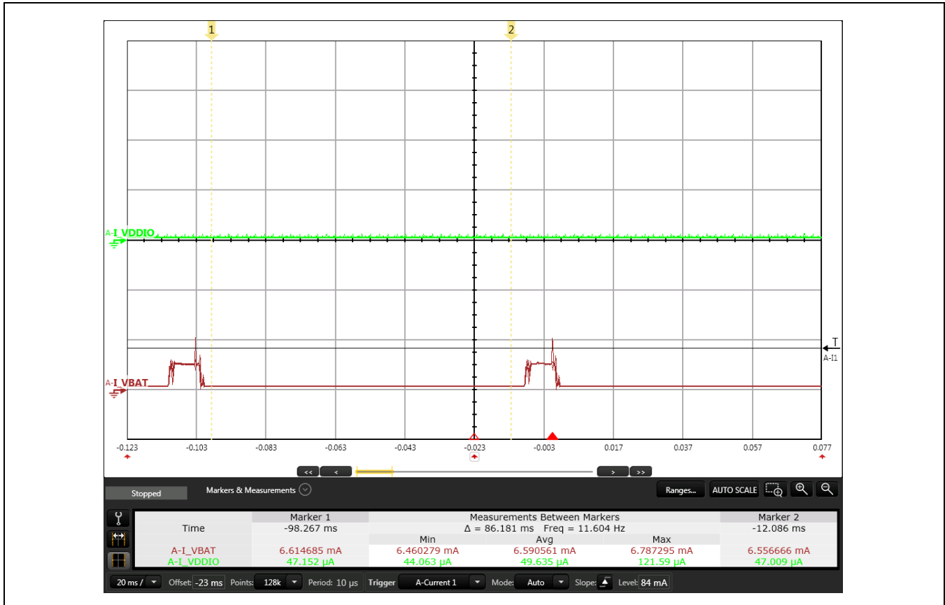
Figure 14. Current—Active Waiting for Packets (IEEE Power Save Mode Enabled, WLAN = Deep Sleep)
