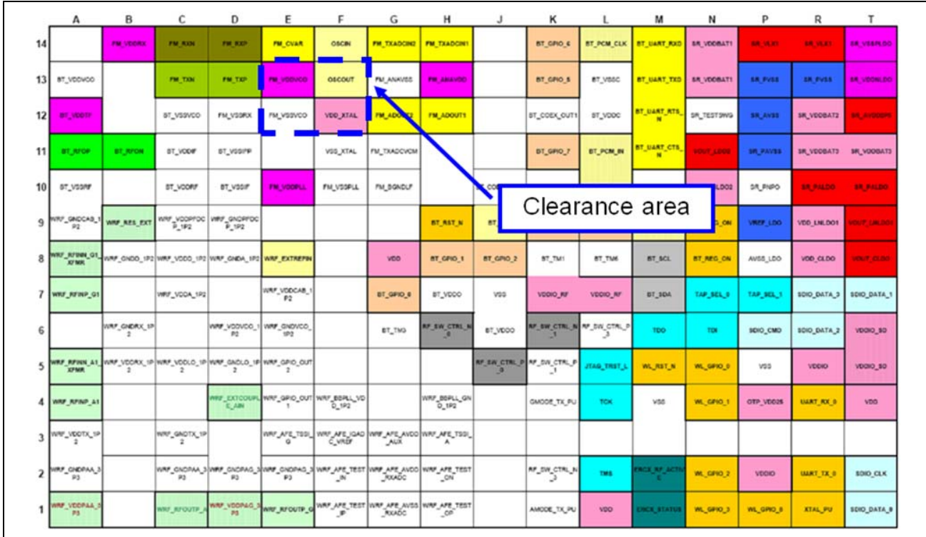
Figure 7: Clearance Area Under the CYW4329
