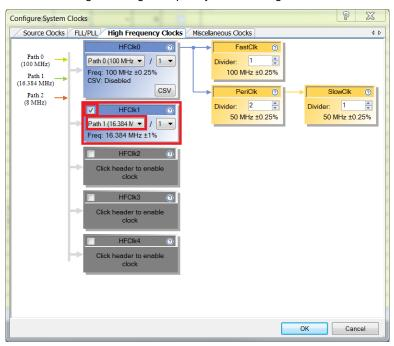
Figure 5. High Frequency Clock Configuration
