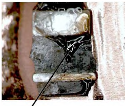
Figure 9 Flux residue compromising isolation
