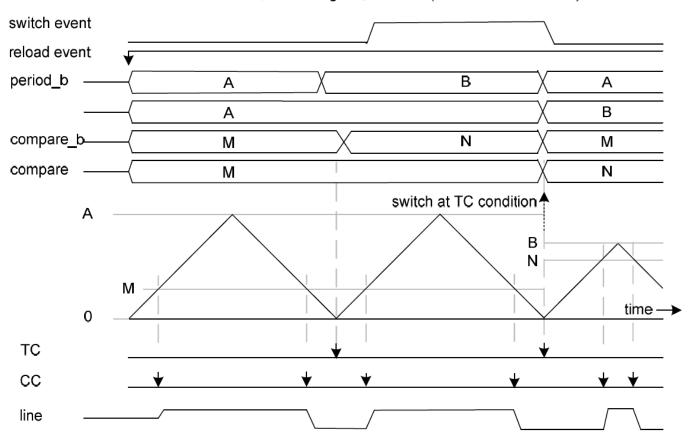
PWM, center aligned, buffered (software switch event)
