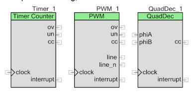
The base component in the catalog is setup in the unconfigured mode. The unconfigured component is configured at run-time through function calls to perform the operation of any of the modes.
