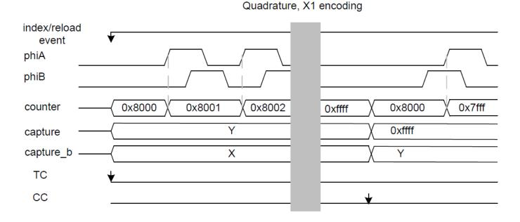
When the counter reaches "0xFFFF" (the maximum counter value), the counter value is copied to the capture register and the counter is initialized to "0x8000" (the mid-point counter value). A CC condition is generated when the counter value is copied. This condition can be used to generate an interrupt.
