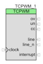
component as an unconfigured TCPWM and the specific configuration setup at runtime with the API interface.
