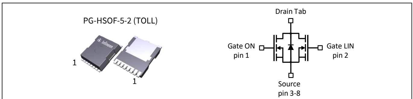
Figure 7 Dual Gate MOSFET TOLL package and equivalent circuit symbol
