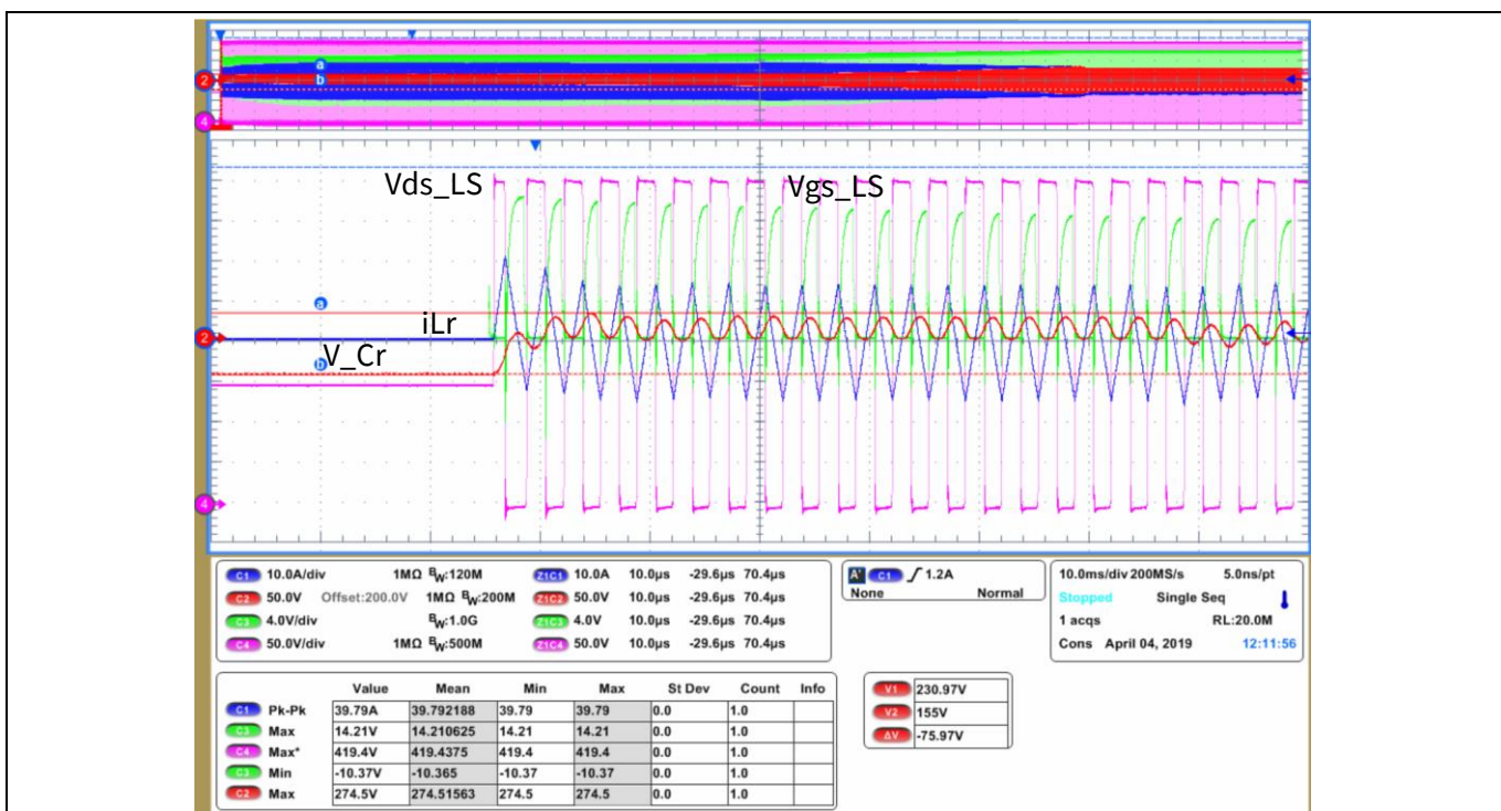
Figure 47 C r during start-up at nominal input 400 V and nominal output 51.5 V.
