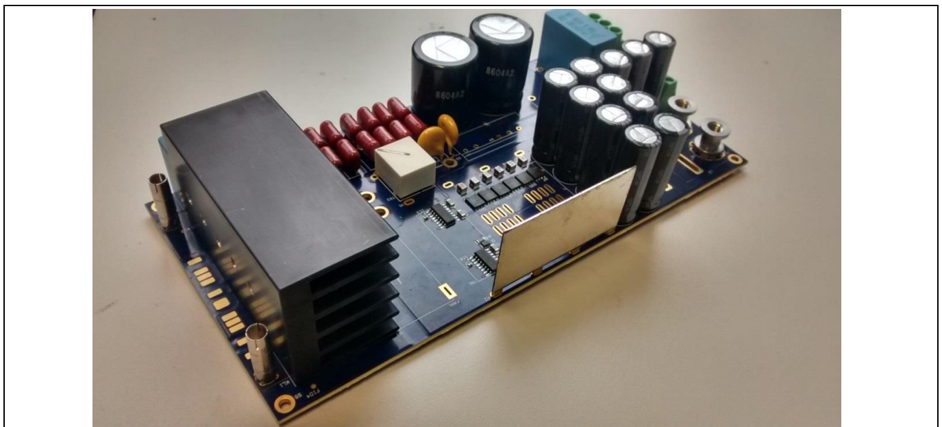
Figure 29 Heatsinks for HV HB devices and LV secondary devices in a partially assembled 3300 W LLC HB converter board
