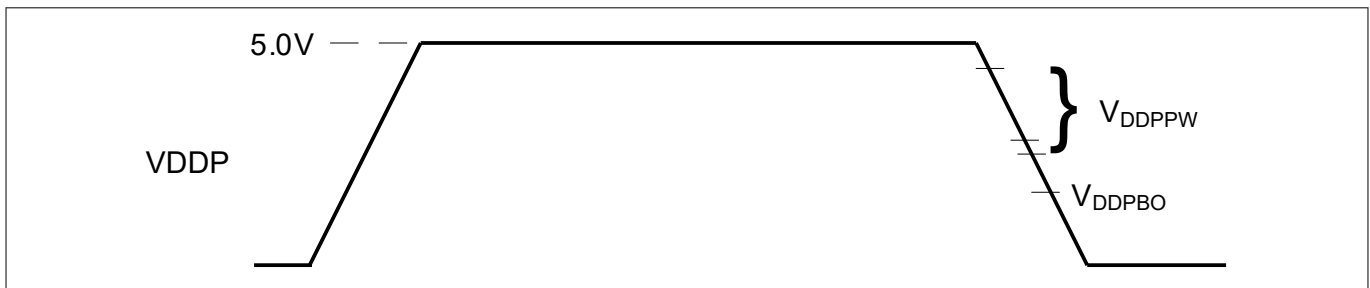
Figure 17 Supply Threshold Parameters
