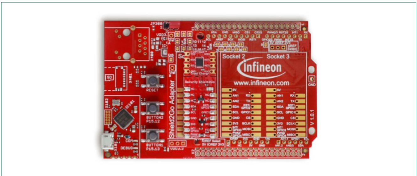
Figure 6 Infineon’s evaluation kit speeds up the process of designing authentication for wireless charging
