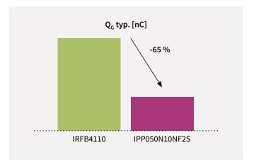
Compared to the previous StronglRFET<sup>TM</sup> generation in 100 V TO-220 package, StronglRFET<sup>TM</sup> 2 shows significant improvements such as  $\sim$ 40 % lower R<sub>DS(on)</sub> and  $\sim$ 65% reduced Q<sub>G</sub>. This results in better efficiency and longer life time.
