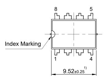
1) Does not include plastic or metal protrusion of 0.25 Max. per side All dimensions are in units mm
