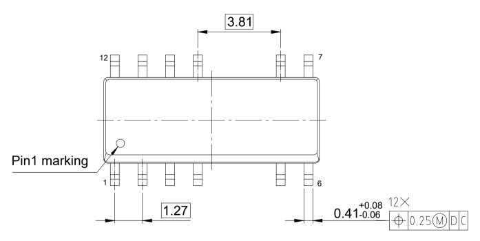
1) Does not include plastic or metal protrusion of 0.25 max. per side All dimensions are in units mm
