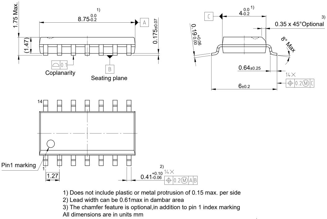
The drawing is in compliance with ISO 128-30, Projection Method 1 [ $\bigcirc$ ] Drawing according to ISO 8015, general tolerances ±0.05; ±30'
