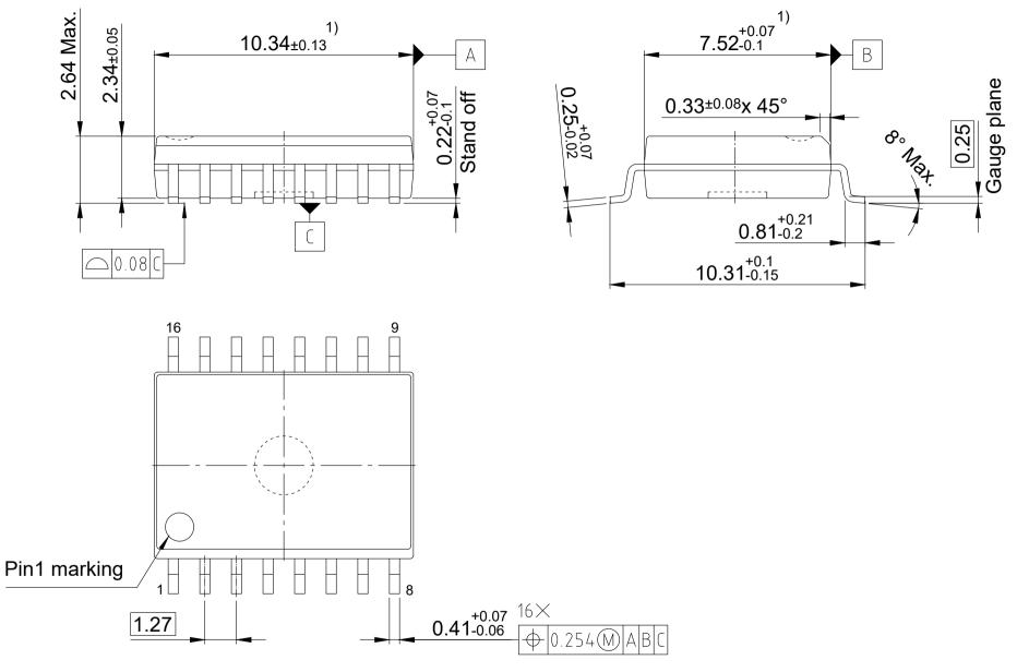
1) Does not include plastic or metal protrusion of 0.15 max. per side All dimensions are in units mm
