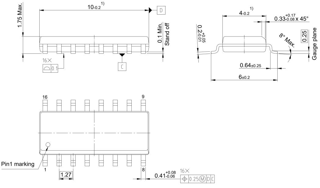
1) Does not include plastic or metal protrusion of 0.15 max. per side All dimensions are in units mm
