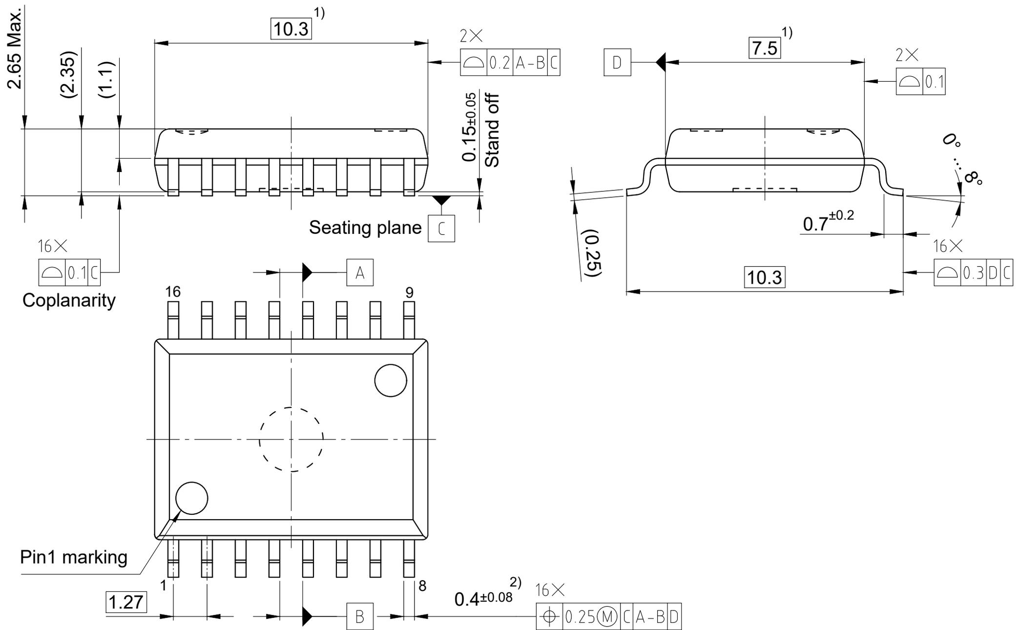
1) Does not include plastic or metal protrusion of 0.15 max. per side
