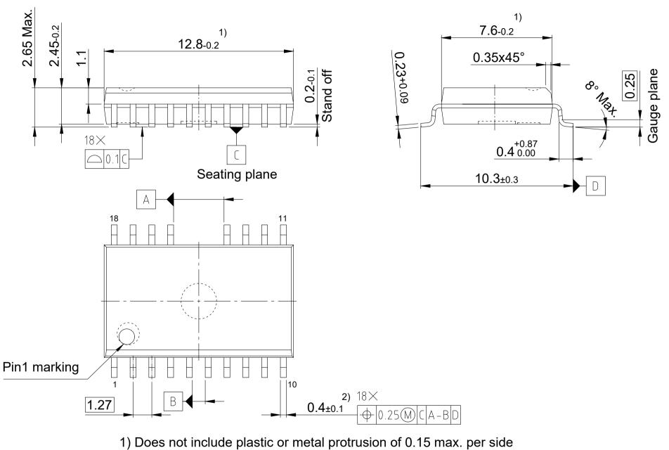
2) Does not include dambar protrusion of 0.1 max.
