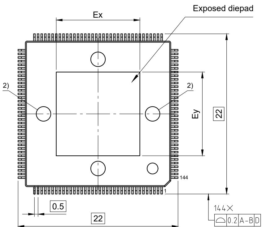
1) Does not include plastic or metal protrusion of 0.25 max. per side
