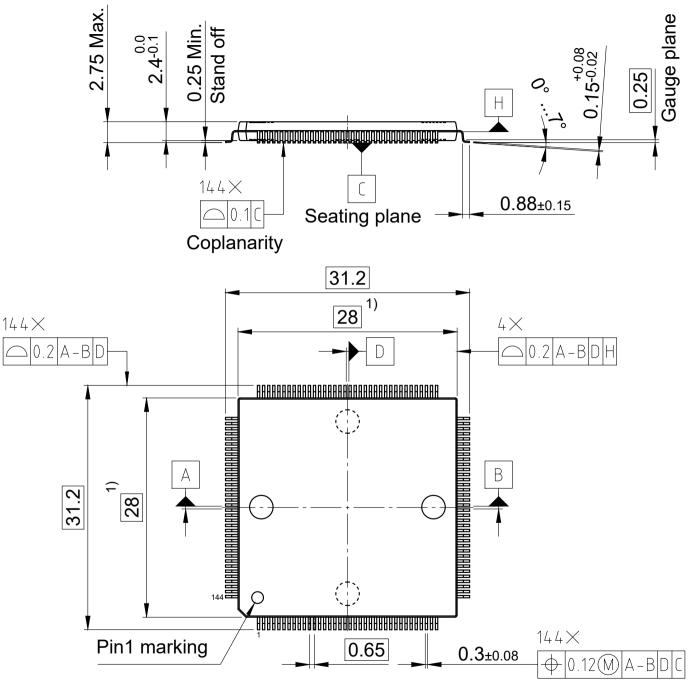
1) Does not include plastic or metal protrusion of 0.25 max. per side All dimensions are in units mm
