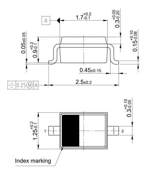
Mold flash, protrusion or gate burrs of 0.15mm maximum per side are not included All dimensions are in units mm
