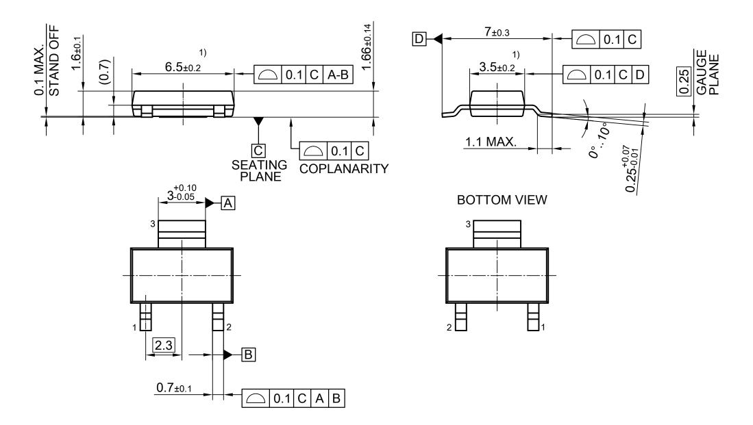
1) DOES NOT INCLUDE PLASTIC OR METAL PROTRUSION OF 0.15 MAX. PER SIDE ALL DIMENSIONS ARE IN UNITS MM THE DRAWING IS IN COMPLIANCE WITH ISO 128 & PROJECTION METHOD 1 [
