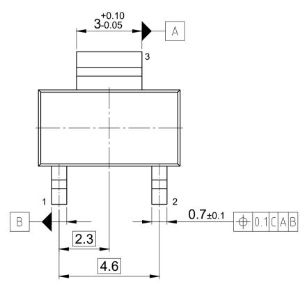
1) Does not include plastic or metal protrusion of 0.15 max. per side All dimensions are in units mm
