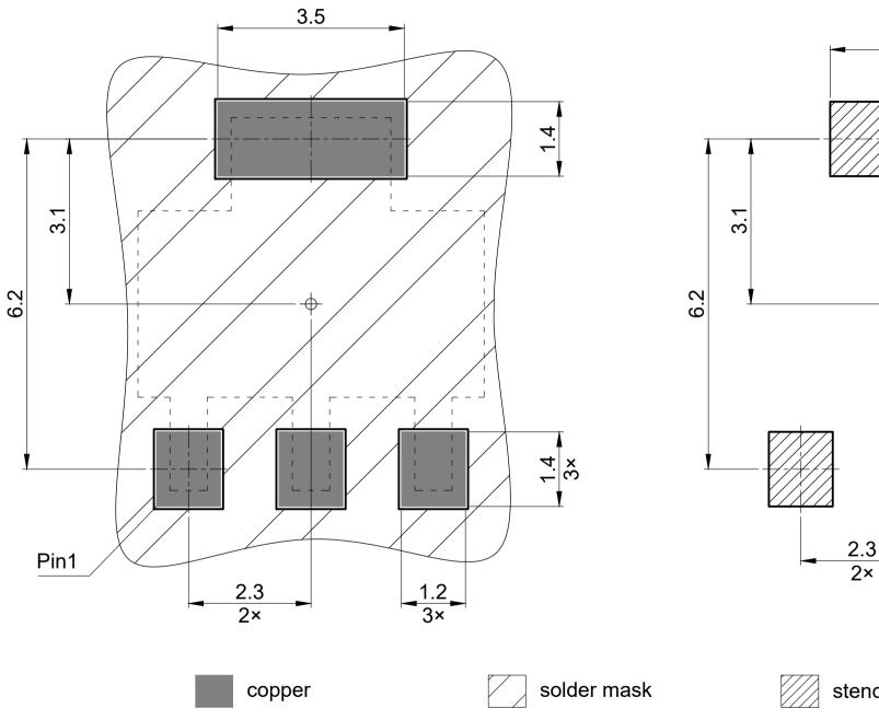
All dimensions are in units mm All pads are non-solder mask defined stencil apertures
