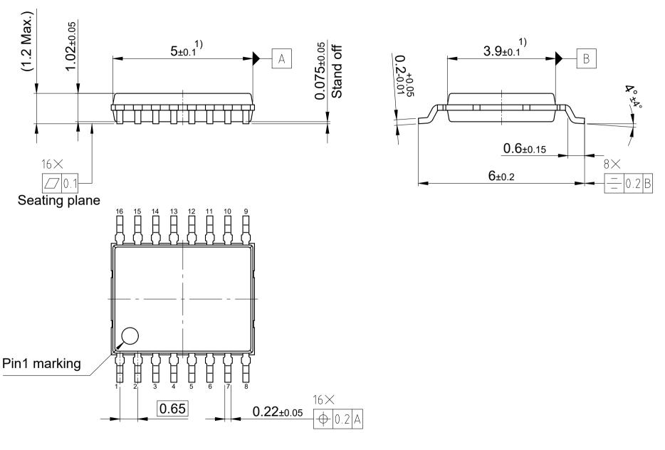
1) Outer dimension does not include protrusion or intrusion of 0.15 per side All dimensions are in units mm
