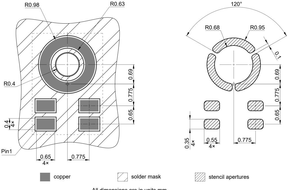
All dimensions are in units mm All undimensioned radii is 0.1mm All pads are non-solder mask defined
