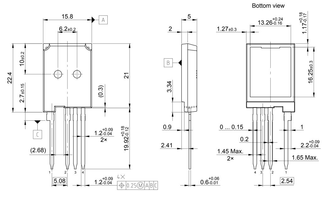
All dimensions refer to JEDEC standard TO-247 and do not include mold flash or protrusions. Pkg surface route between pin 1 & pin 2 will be 5.1mm min.
