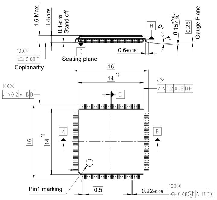
1) Does not include plastic or metal protrusion of 0.25 max. per side All dimensions are in units mm
