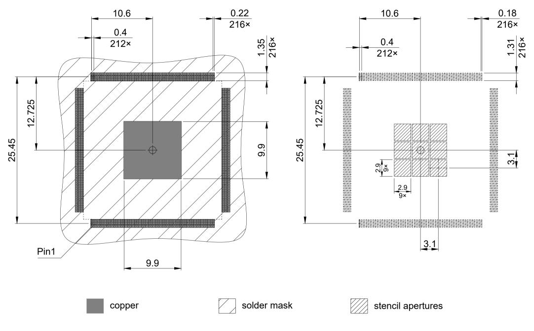
All pads are non-solder mask defined All dimensions are in units mm
