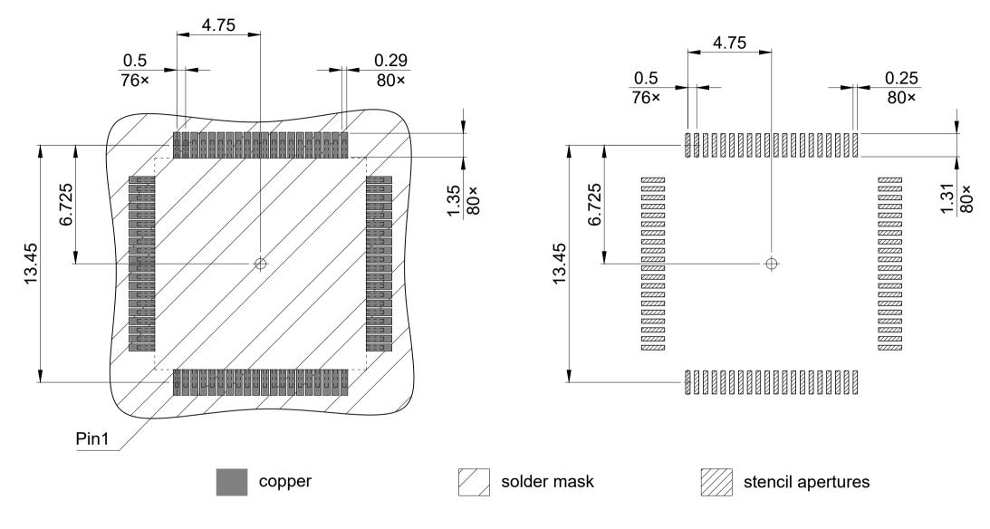
All pads are non-solder mask defined All dimensions are in units mm
