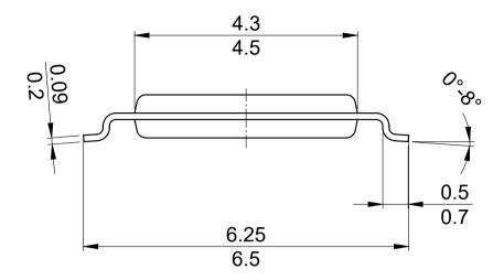
All dimensions are in units mm  $\frac{\text{min.}}{\text{max.}}$
