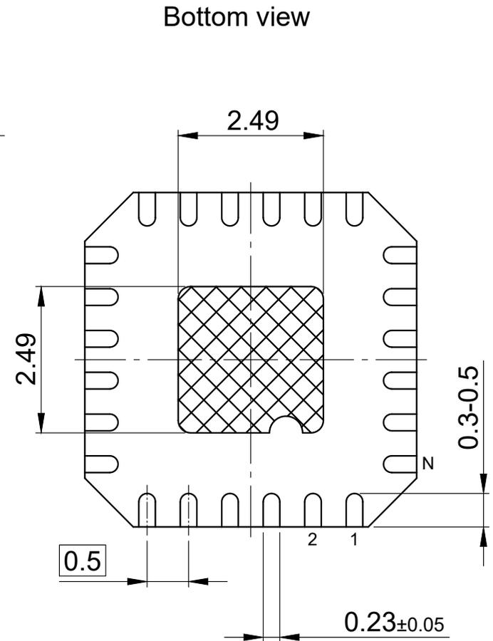
▣ Hatch is solderable exposed metal.
