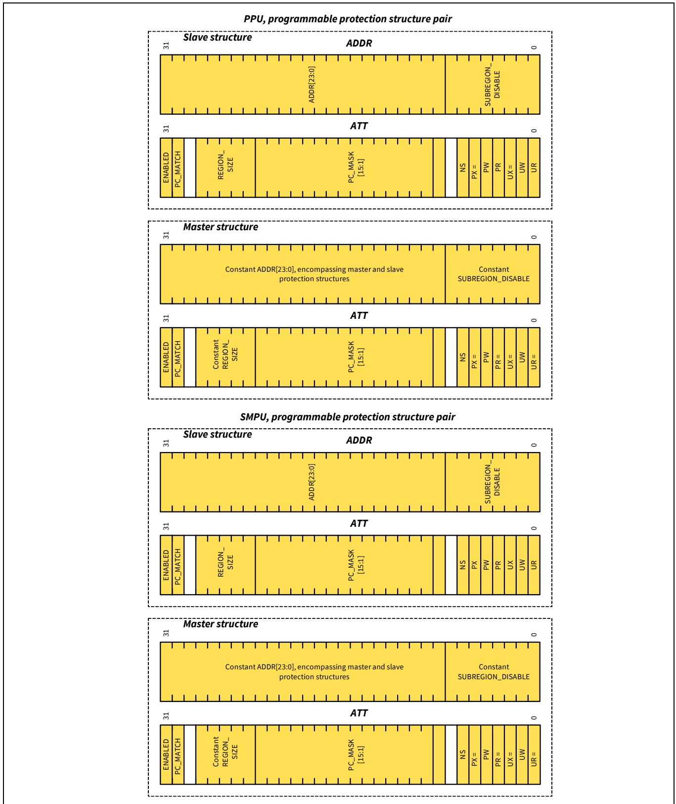
Figure 9-7. Programmable protection structure pair
