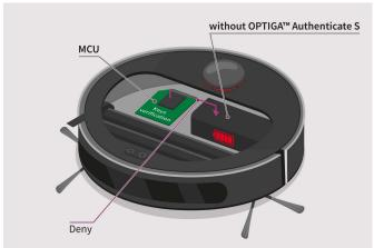
A counterfeit battery may compromise the safety of the robot. With OPTIGA™ Authenticate S, it is possible to check whether replacement parts like batteries are genuine.
