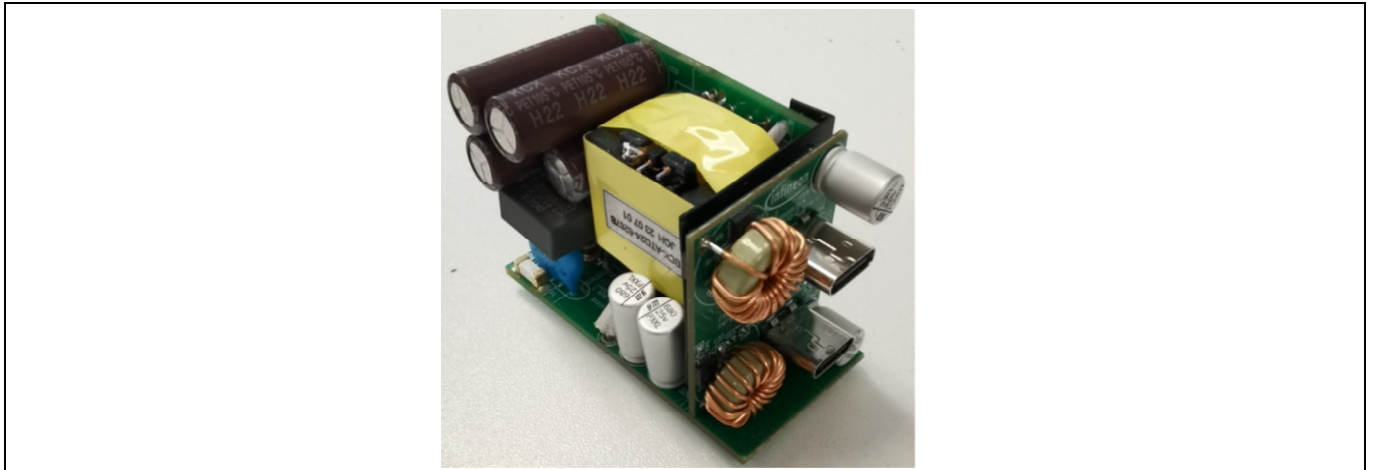
Figure 2 REF_65W_2C_GAN_PAG1 + CCG7DC 65W_2C with ATQ solution board
