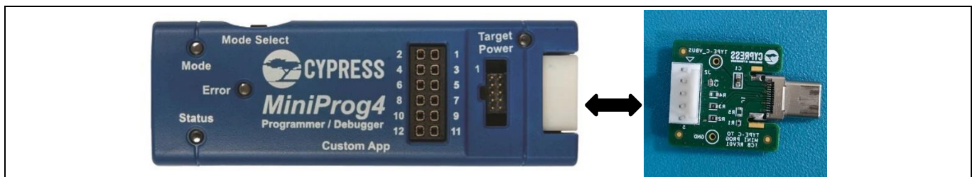
Figure 4 PSoC™ MiniProg4 (CY8CKIT-005) Programmer Kit
