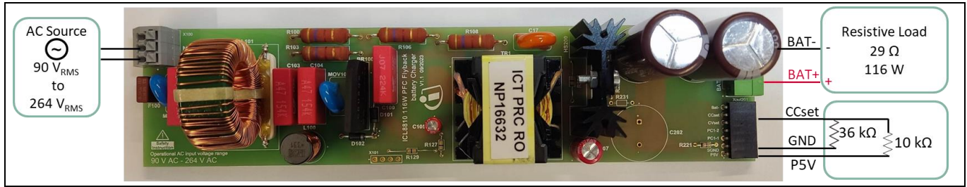
Figure 3 EMI test setup with full output power
