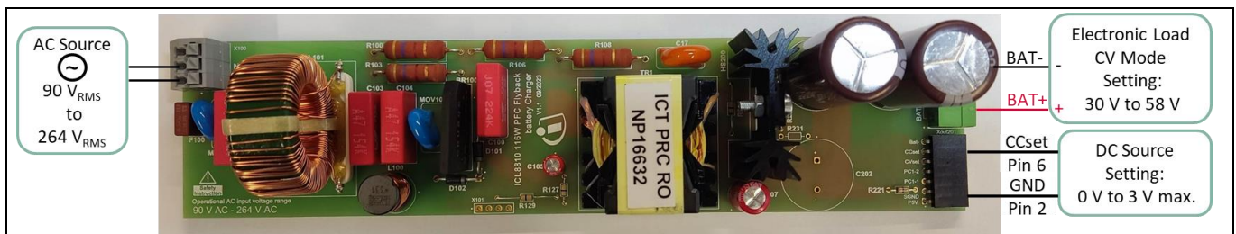
Figure 2 Test setup with electronic load and adjustable CC set point using DC source
