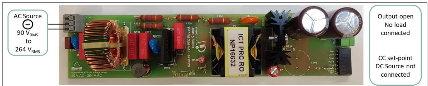
Figure 4 No-load system standby power test setup
