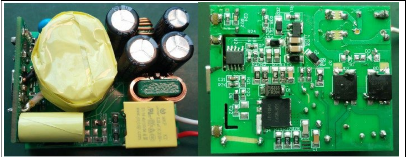
Figure 13 A 65 W reference design using PAG1S and PAG1P in a 52 mm x 42 mm x 22 mm board
