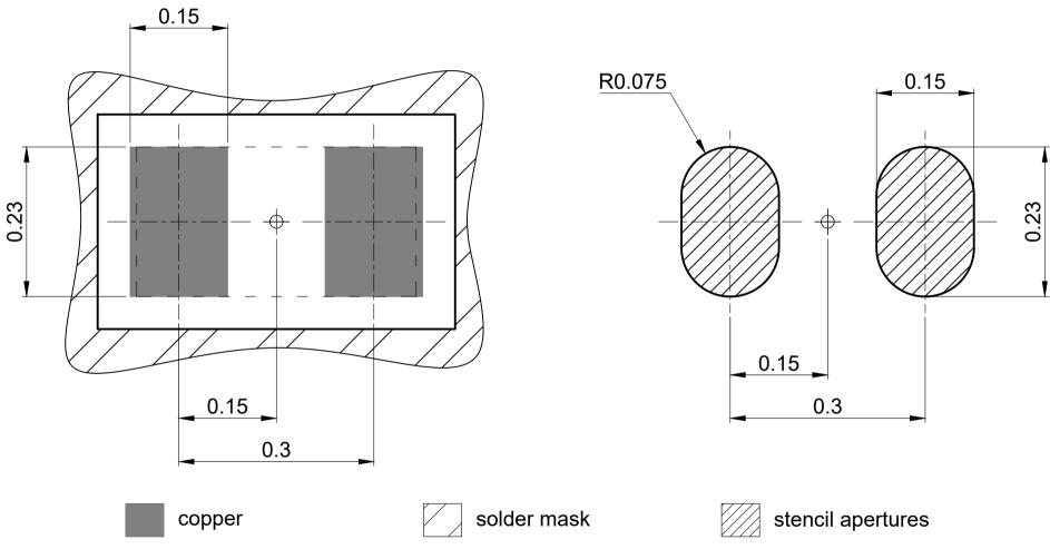
Based on stencil thickness 0.06 mm All dimensions are in units mm
