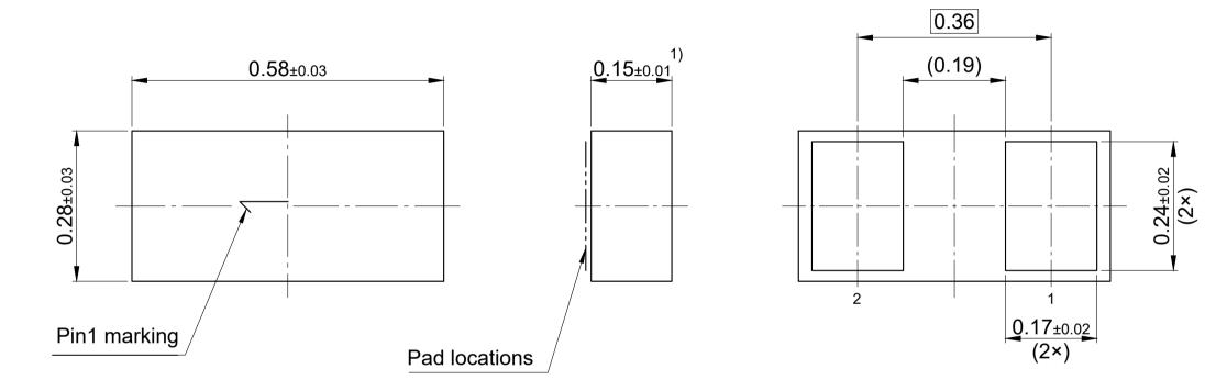
1) The total package height includes the pad thickness
