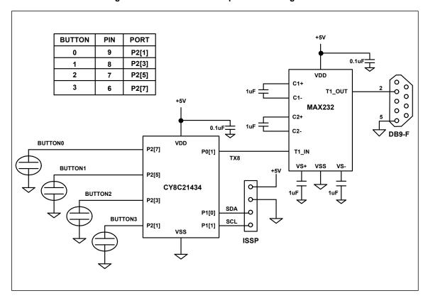
Figure 5. Schematic for the capacitive sensing circuit
