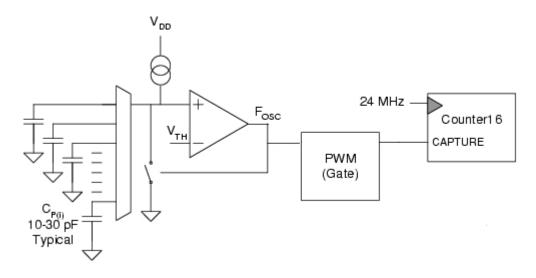
The output of the comparator is fed into the clock input of a PWM which gates a 16-bit counter clocked at 24MHz. A finger on the sensor increases the capacitance, thus increasing the counts. This is how a finger is sensed. Typical waveforms for this system are shown in figure 4.
