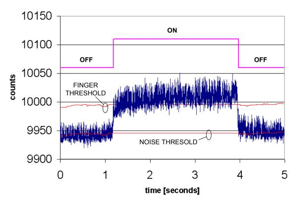
Figure 8. Measured performance of the sensor through 10mm of glass
