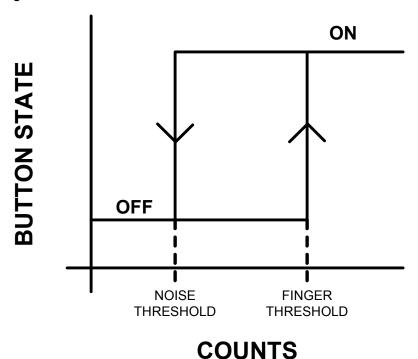
An idealized raw counts waveform for a 3 second button press is shown in figure 7. The threshold levels for this project are shown in the figure. The Noise Threshold is set to 10 counts, and the Finger Threshold is set to 60 counts. The noise component that is always present in real count data is not shown in figure 8 so that the threshold levels can be seen clearly.
