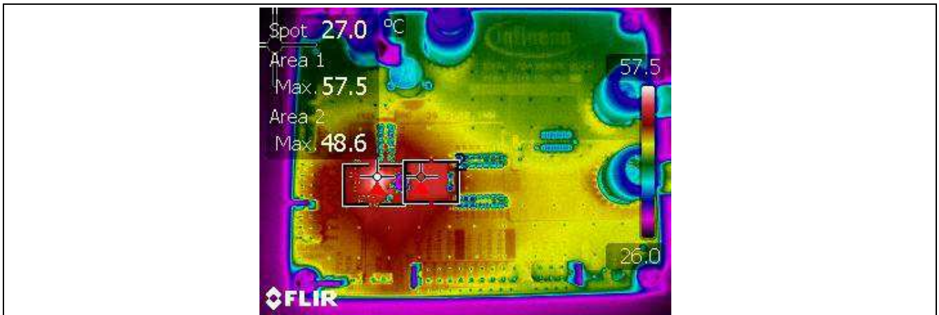
Figure 22 Thermal image at 20 A load TDA38820 = 58°C, L = 49°C, f_{sw} = 600 kHz, T_a = 25^\circ\text{C} , natural convection
