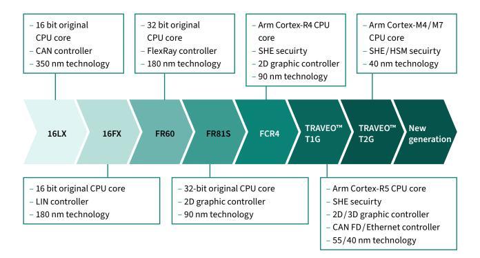
The architecture of TRAVEO™ Microcontrollers has been actively shaped with 30 years of experience gained by building 5 predecessor MCU series built for the automotive segment.
